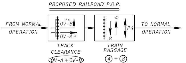
\*OV-A SHALL BE PROGRAMMED FOR THE FAR SIDE EASTBOUND SIGNAL HEADS. PROVIDE 2 SECONDS OF TRAILING GREEN EXTENSION ON OV-A.
