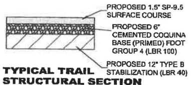
TYPICAL TRAIL STRUCTURAL SECTION STA. 95+08.70 TO STA. 96+34.99 STA. 96+66.72 TO STA. 96+96.02
