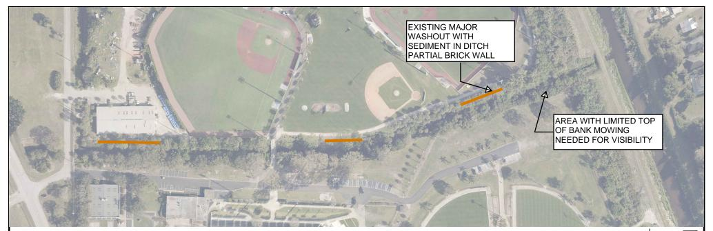
CLEARING WORK SHALL BE PERFORMED PRIMARILY FROM WITHIN THE CANAL AND THE WESTERN BANK. HEAVY EQUIPMENT WILL NEED TO ENTER AND EXIT THE CANAL AT EACH CROSSING WHICH MAY IMPACT THE BANK AND REQUIRE MINOR REPAIR. VEGETATION REMOVAL MAY NOT OCCUR IN AREAS WHERE THE BANK IS DESTABILIZED IN ITS EXISTING CONDITION TO MINIMIZE ANY FURTHER DAMAGE.
