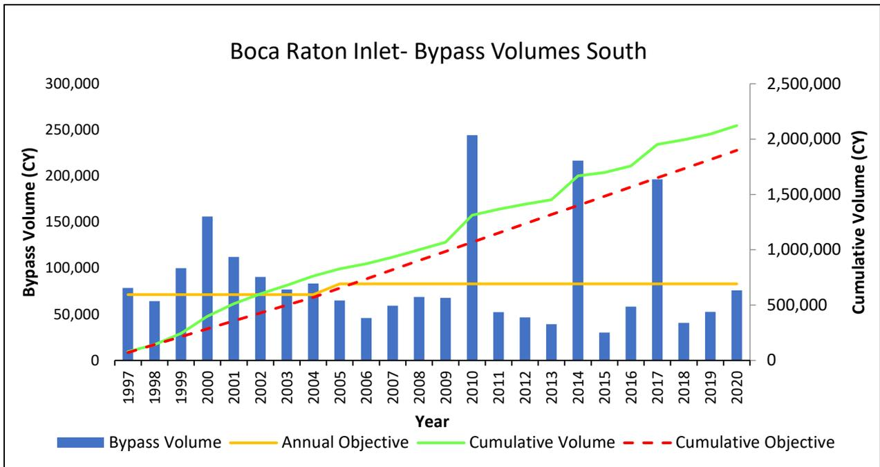
**Figure 17:** Boca Raton Inlet bypass volume, annual objective, cumulative volume and cumulative objective.
