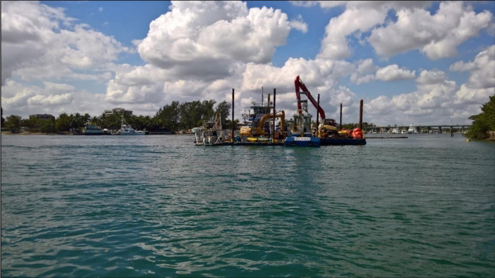
**Figure 13:** Jupiter Inlet with the Cavache Dredge working within the inlet to bypass sand, March 2017. Photo by Libbie McDermid (DEP) in March 2017.
