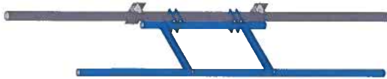
1 S-3 STANDOFF MOUNT INSTALLATION ISOMETRIC VIEW NTS
