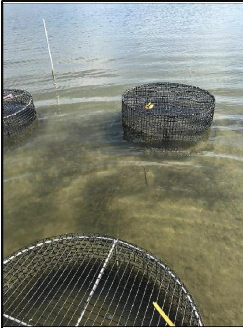
Figure 3. GrowSAV™ Herbivory Exclusion Devices deployed on 15-foot centers in a cluster of five marked with PVC poles.
