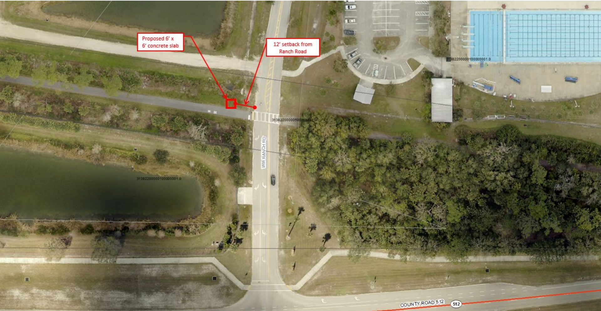
Map of bicycle repair station location with proposed 6'x6' concrete slab 12' setback from Ranch Road.
