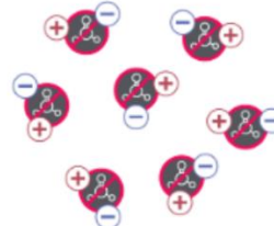
Oxygen ions cause a chemical reaction with VOCs breaking down their molecular structure
