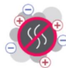
Odorous gases and aerosols oxidize on contact with oxygen ions and are neutralized
