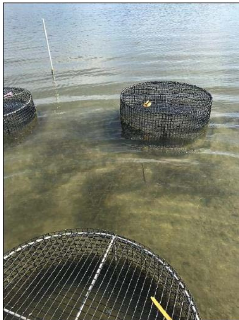
Image 1. GrowSAV™ Herbivory Exclusion Devices deployed on 15-foot centers in a cluster of five marked with PVC poles.
