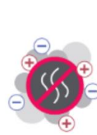
Odorous gases and aerosols oxidize on contact with oxygen ions and are neutralized
