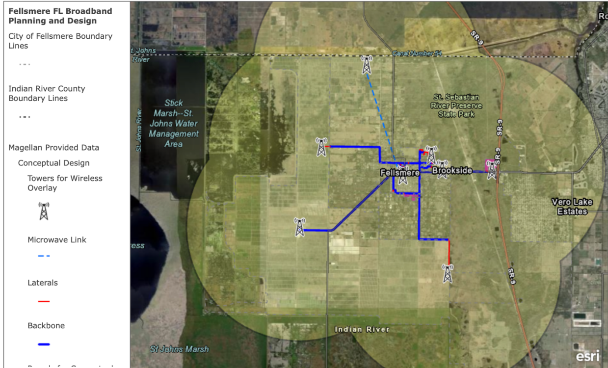
Figure 15: Fellsmere Design and Towers for Wireless Network
