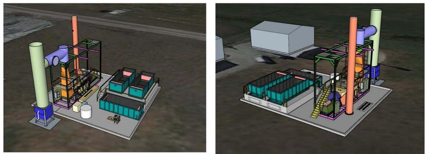
Figures D-2 and D-3. Illustration of facility layout, with enclosed Flare and two roll-off boxes.
